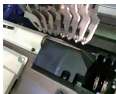
剪刀清洁装置：自动清除剪刀夹子的线头 The clean system within cutter: Automatic clean the yarn debris within the cutter
